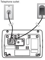
Plug one end of the telephone line cord into the telephone line
